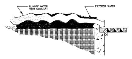
**Figure 7.35-4 Sod Inlet Protection Device**
