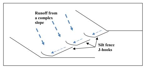
Figure 7.34-1 J-Hook Installation Example
