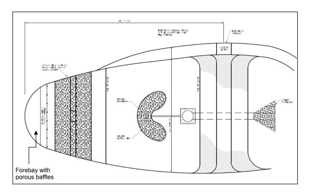
Figure 7.31-2A Sediment Basin with Forebay, Plan View
