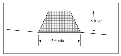
Figure 7.38-1 Filter Berm Dimensions
