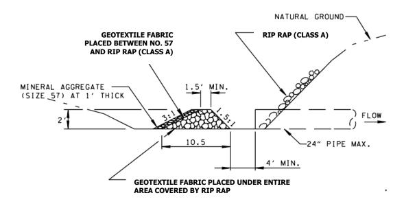
Figure 7.30-1 Filter Ring Detail (Source: TDOT Standard Drawing)
