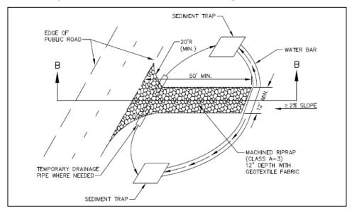
Figure 7.28-1 Construction Exit with Water Bars
