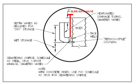
Figure 7.31-8 Slotted Drain Pipe Dewatering Device
