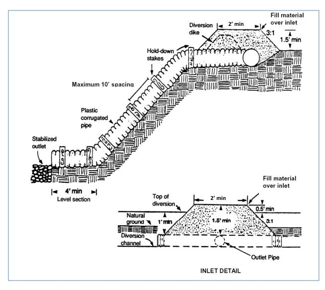
Figure 7.24-1 Slope drain pipe and inlet detail (Source: GA SWCC)
