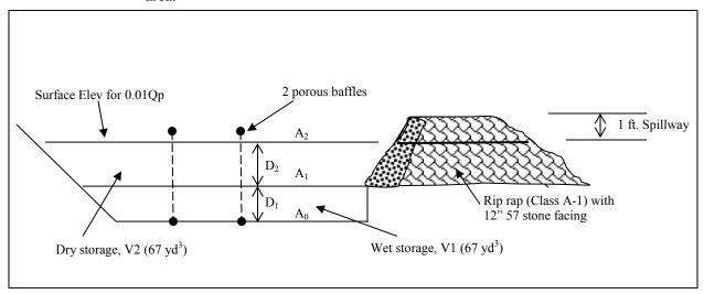
Figure 7.32-1 Sediment trap
