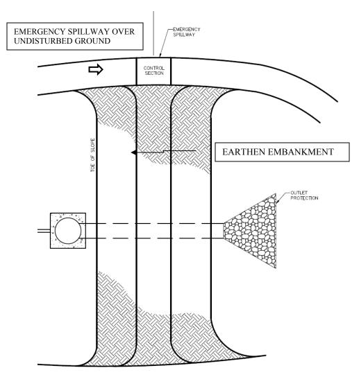
Figure 7.31-11 Earthen Embankment
