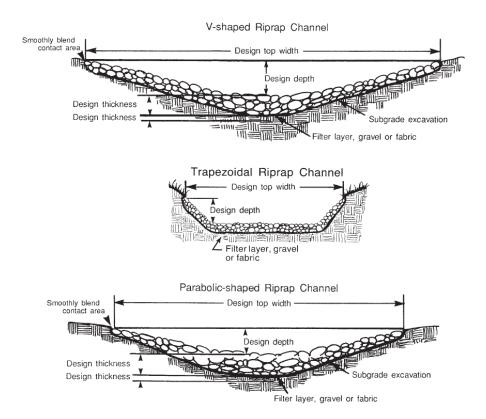
Figure 7.27-6 Construction details for riprap lined channels
