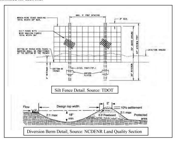
Figure 5.2-1 Typical Construction Detail
