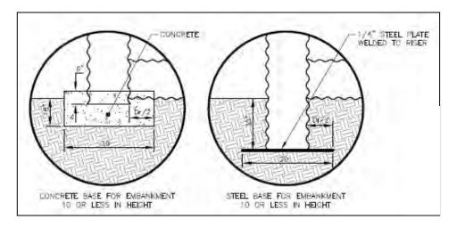
Figure 7.31-4 Anti-Flotation Device
