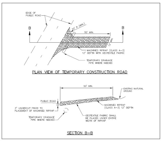
Figure 7.28-2 Construction Exit Detail
