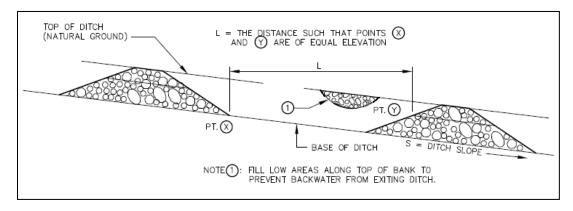
Figure 7.20-2 Spacing between check dams (Source: TDOT)
