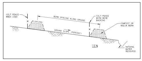
Figure 7.38-2 Mulch Berm with Silt Fence with Backing
