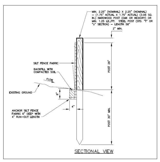
Figure 7.34-2 Silt fence details
