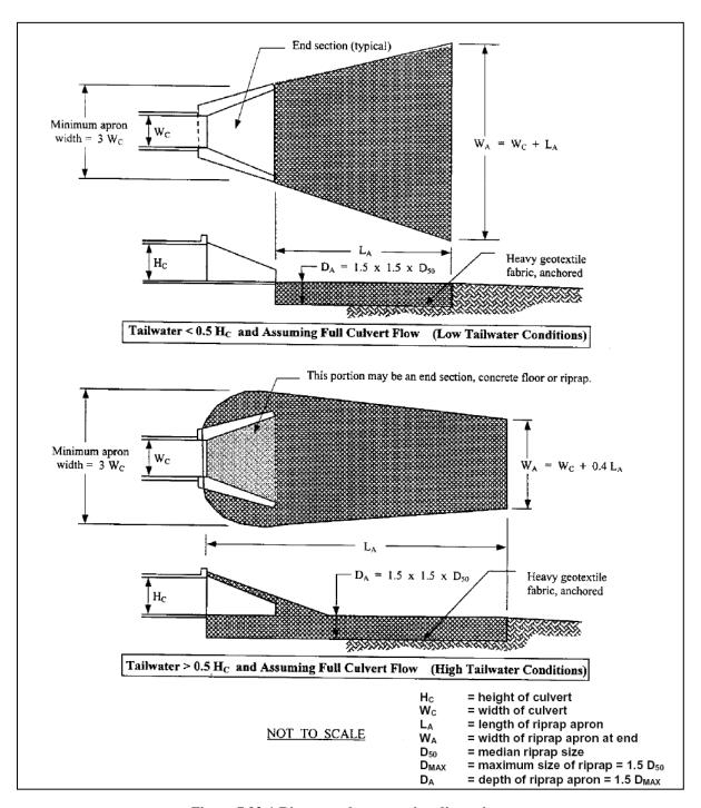
Figure 7.23-1 Riprap outlet protection dimensions (Knoxville Engineering Department)
