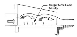
Typical Energy Dissipator - Baffle Blocks Within Headwall
