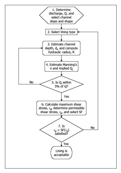
Figure 7.27-1 Decision Flow Chart for Design of Flexible Channel Linings (Source: FHWA HEC 15)
