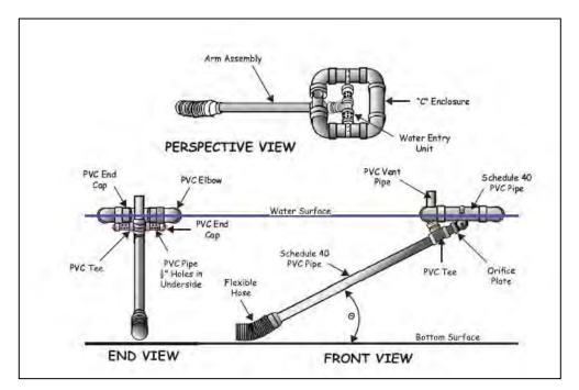
Figure 7.31-9 Schematic of a floating skimmer dewatering device
