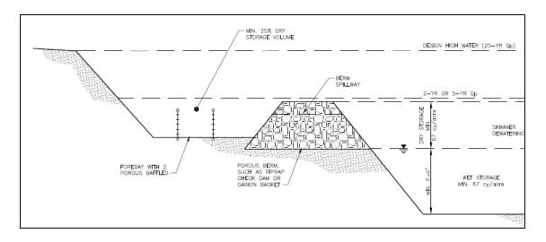
re 7.31-2B Cross Sectional View of Forebay, Showing Elevations
