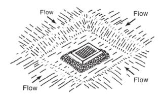
Figure 7.35-1 Excavated Inlet Protection (Source: NCDENR)
