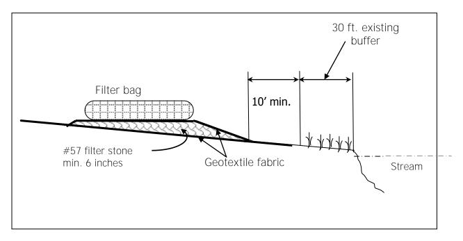
Figure 7.21-2 Sediment filter bag
