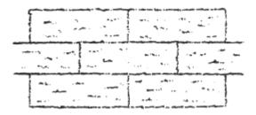
Figure 7-7.10-1. Correct sod placement
