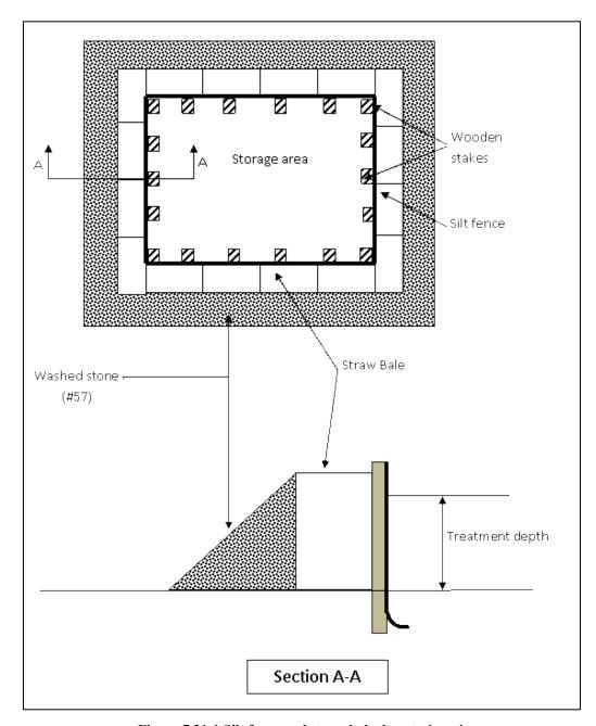
Figure 7.21-1 Silt fence and straw bale dewatering pit
