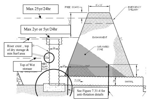
Figure 7.31-3 Elevations within the Basin
