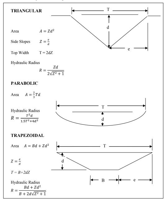
Figure 7.27-2 Channel Geometry, Cross-sectional Area and Hydrologic Radius
