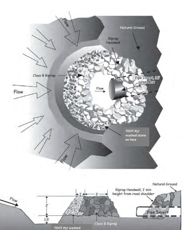
Figure 7.35-5 Rock Pipe Inlet Protection (Source: NCDENR)
